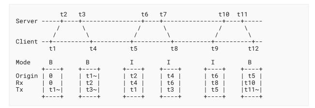
Figure 1: Packet Timestamps in Interleaved Client/Server Mode
